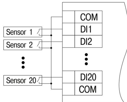
Fig. 4.5 Connection to the inputs DI1–DI20 (MV210-204)
