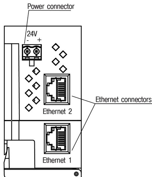
Fig. 4.1 Device's connectors
