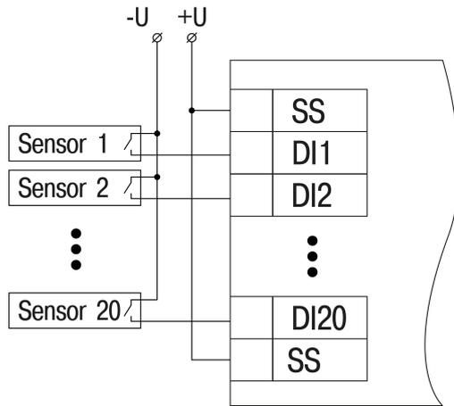
Fig. 4.4 Connection to the inputs DI1–DI20 (MV210-202)
