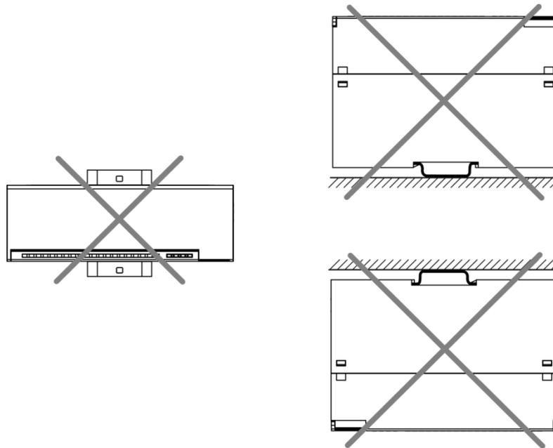
Fig. 3.2 Improper installation
