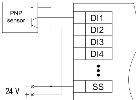
Fig. 4.6 Connection of PNP transistors (only for MV210-202)
