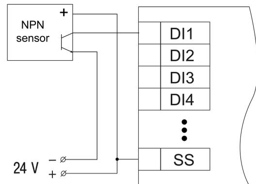
Fig. 4.7 Connection of NPN transistors (only for MV210-202)
