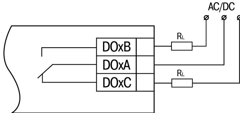
Fig. 4.5 External connections to the outputs with changeover contacts
