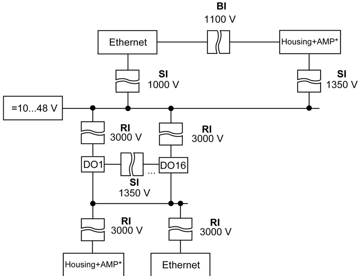
Fig. 2.1 Isolation of the Device Components
