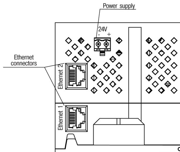
Fig. 4.2 The device's connectors
