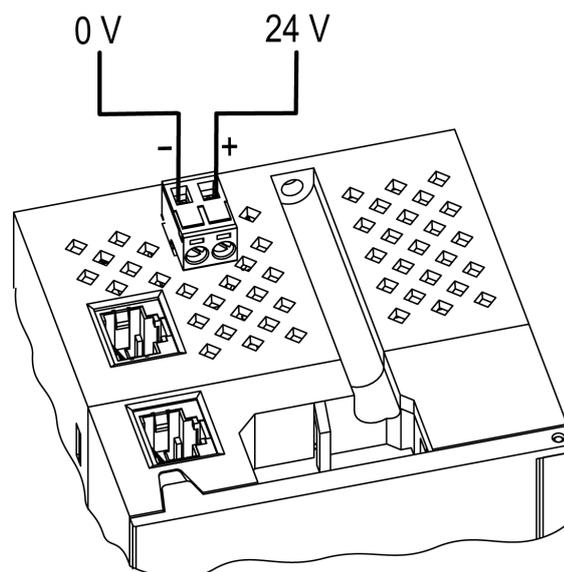
Fig. 4.3 Power supply contacts function
