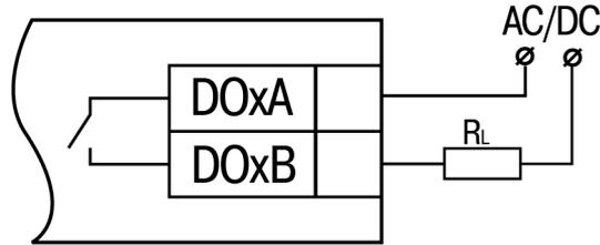
Fig. 4.4 External connections to the outputs with normally open contacts
