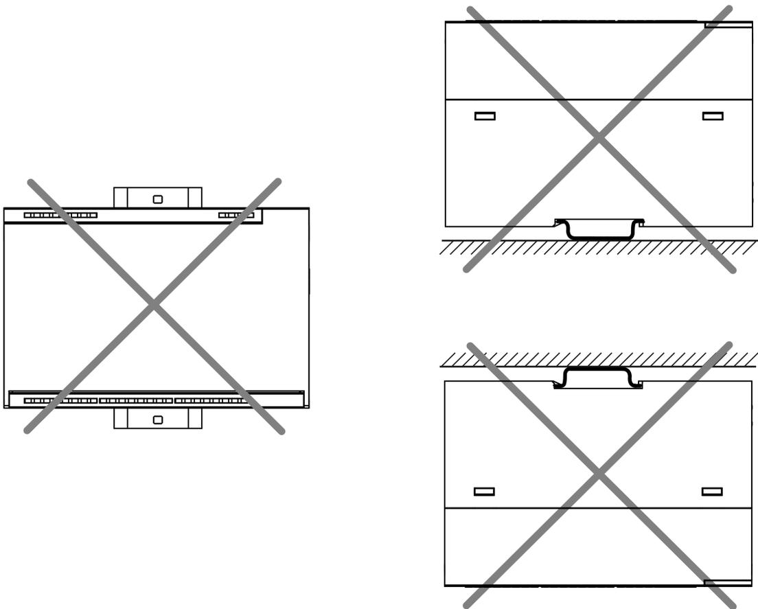
Fig. 3.2 Improper installation
