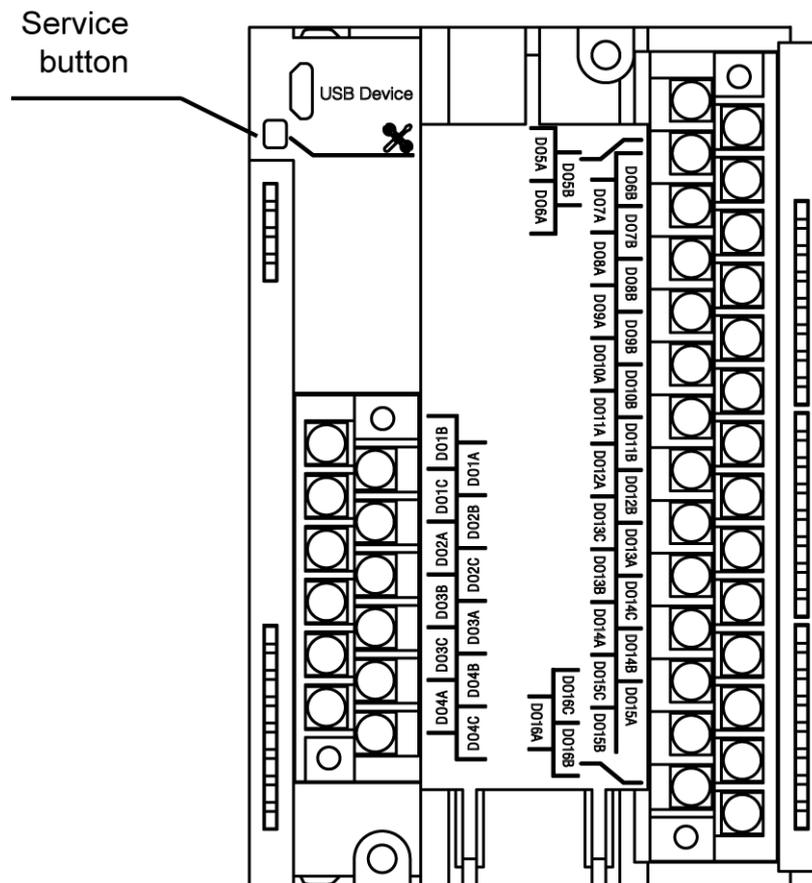
Fig. 4.1 Terminal block layout
