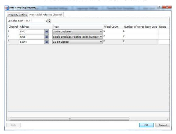
It can be seen that the sampling addresses of multiple channels could be non-continuous addresses.
