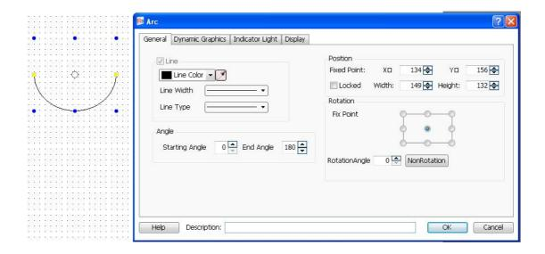
An arc can be got by setting the properties such as line color, width, type, starting angle, end angle, position and rotation. It can be freely drawn by dragging the yellow and blue areas.
