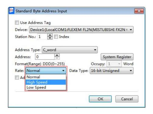
Certainly, you can use the address tag library. You need to prepare the data addresses in the address tag library before using them. Check the "Use Address Tag" in the "Standard Byte Address Tag" window and click the button "[Standard Byte Address Tag" window and click the button "Tag Library" window. Select the byte or word address you need in the address tag library, as shown as follows.
