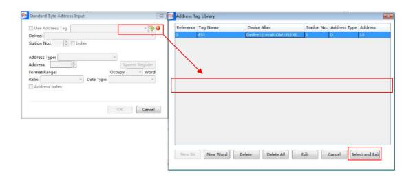
You can use the Address Index function. This function can change the byte or word address which is connected with the current component according to the value of a word address. For example, the word address D0 is connected with the current component. If you check the Address Index and set the address as LW0, as shown as below, the word address which is connected with the current component will beD (0 + LW0).
