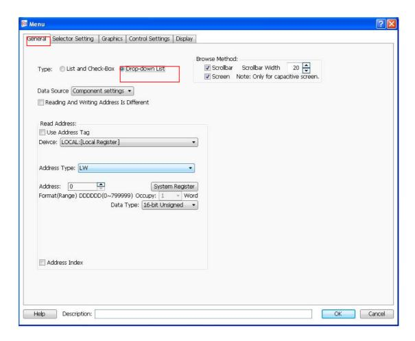
The figure above shows that the "General" property TAB is same to the "Check list and selection boxes", it is not introduced here, and details can be seen in <a href="Detailed">Detailed</a> manual/Commponent/Toggle Switch and menu/Check list and selection boxes.
