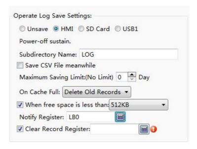
This settings is the global settings, the operating steps can be recorded without setting the operate log control, the default is "unsave", you can choose to save to the local HMI, SD card, USB1. The address of storing operate log is retained after power down, you can define the subdirectory name by yourself. The files saved is Db files.
