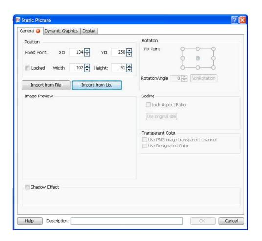
Local picture in the computer or in the software picture library can be imported by clicking the "Import from File" button or the "Import from Lib" button. And the picture will be put into the window by clicking the "OK" button.
