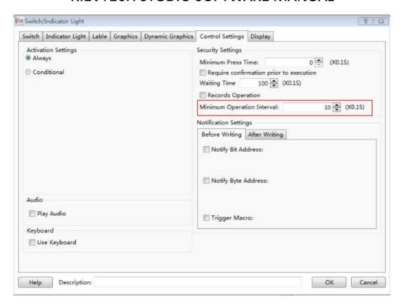
By using the "Minimum Operating Interval" function, continuous actions can be avoided in a short time due to touching the screen continuously by mistake.
