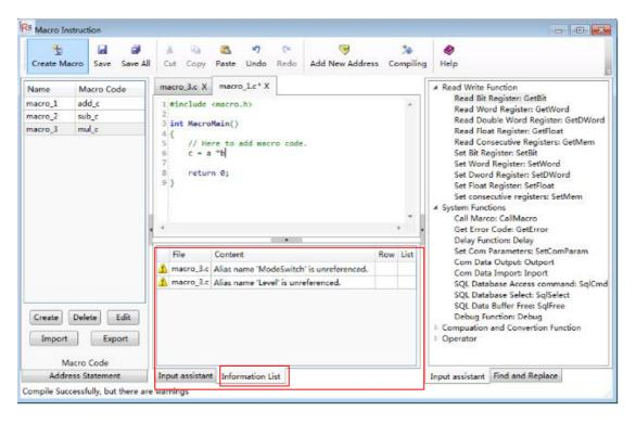
Information List window displays prompts and error messages when the macro compile. You can double-click the error message entryin the list if compiling errors occur. It will quickly navigate to the position where this error occurs.
