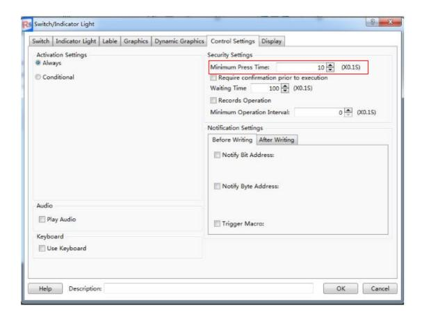
You need to hold the button component for a specified time to perform actions. The function is used to avoid the action due to touching the screen by mistake.
