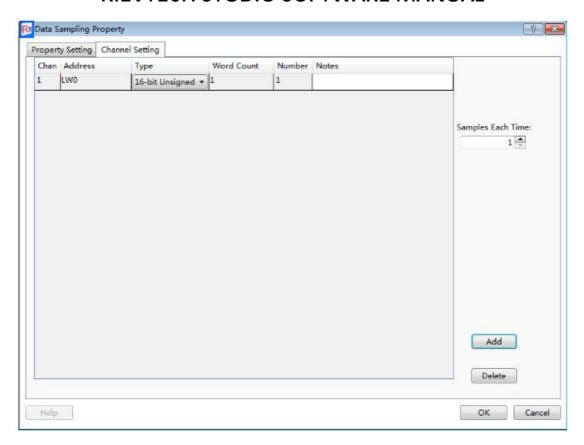
The "Address" refers to the start address of the data record. The "Type" of data record can be "16-bit Unsigned", "16-bit Signed", "32-bit Unsigned", "32-bit Signed", "16-bit BCD", "32-bit BCD", "Single-precision Floating-point Number" or "Character String". The maximum memory occupied is 64 word registers for the type of "Character String".
