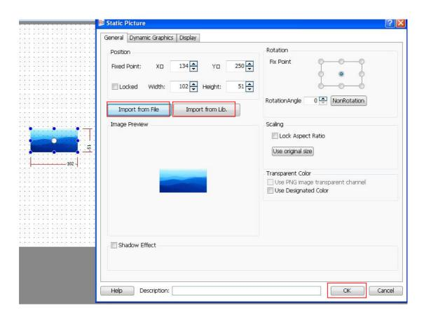
The static picture position can be modified. You can change the position by manually dragging or by setting the coordinates in the static picture properties window. The static picture size can be modified, too.
