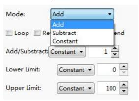
Word setting refers to periodic setting of a word register by timer. The setting modes include "Add", "Subtract" and "Constant".
