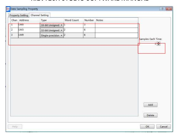
In this example, LW0 ~ LW2 is occupied by the first channel, LW3 ~ LW8 is occupied by the second channel, and LW9 ~ LW14 is occupied by the third channel. The number of addresses is three times as the number which the "Samples Each Time" is set 1.
