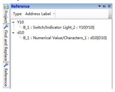
For example, all the uses of "Address" in the current project are listed in the following after selecting it.
