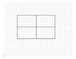
For the fixed-height table, the width and the height of the cells can be modified by mouse-dragging the split line. It is shown as below.
