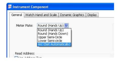
The attributes of the "Round (Hands Up)", "Round (Hands down)", "Upper Semi-Circle" and "Lower Semi-circle" are same. For the Arc Meter Plate, you can freely set the starting angle and ending angle, as shown as below.
