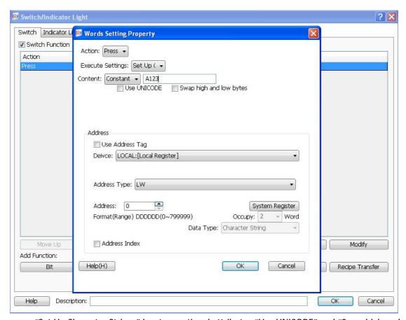
"Set Up Character Strings" has two optional attributes "Use UNICODE" and "Swap high and low bytes". When "Use UNICODE" is checked, it means the character string written to registers is coded by UNICODE. The string is normally displayed only in "UNICODE". If "Swap high and low bytes" is checked, the high and low bytes in the character string will be exchanged before written to the word register.
