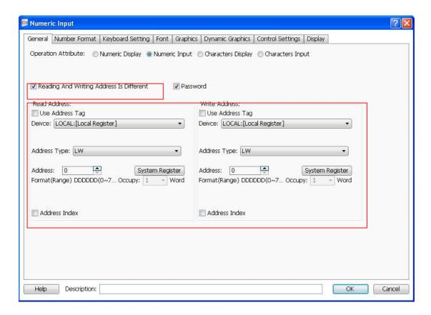
The numeric value input component is integrated with functions of reading data from an address and writing data to an address. When the "Reading And Writing Address Is Different" is not checked, the using method is same to the "Numeric Value Display" component. When the "Reading And Writing Address Is Different" is checked, different address can be set in the "Read Address" and in the "Write Address".
