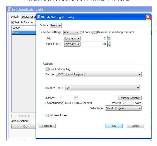
The type of "Execute Settings" includes "Add", "Subtract", "Increase", "Decrease", "Set Up Constants", "Set Up Character Strings", "Set Up Figures By Bit" and "Logic Operation".
