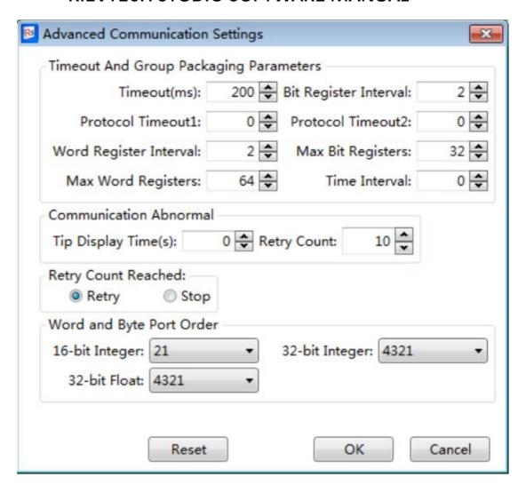
The parameters in the Advanced Communication Settings should not be modified. The optional modification may result in a communication failure or unexpected events occur. You can consult the factory technical staff to modify the advanced parameters based on your needs.
