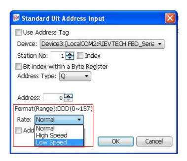
Certainly, you can use the address tag library. You need to prepare the data addresses in the address tag library before using them. Check the "Use Address Tag" in the "Standard Bit Address Tag" window and click the button "Open the "Address Tag Library" window. Select the bit address you need in the address tag library, as shown as follows.
