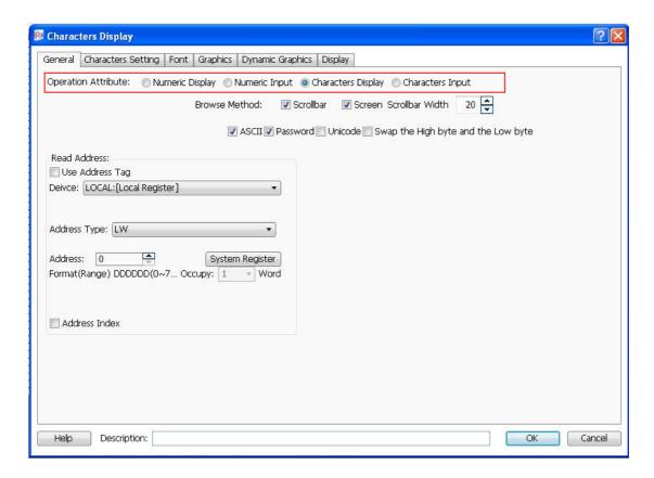
The "Operation Attribute" includes four operation types: "Numeric Display"," Numeric Input", "Character Display" and "Character Input". If you want the current Character Display component change to the Character Input component or Numeric component, you can modify it here. It is highly efficient for the project modifying and maintaining.
