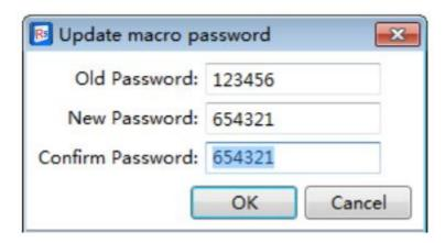
Enter the correct old password and valid new password, then clicking the button "OK" to confirm the password modification.
