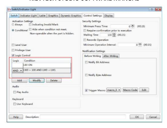
There is a relationship option in front of the second condition in the Logic Control list. The option can be set "AND" or "OR". It means the logic relationship between the previous condition and the following condition. The component can be operated or display only if the result of all the conditions logic operation is true.
