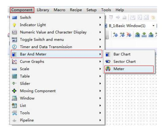
You can add a Meter component by clicking the corresponding tool button in the shortcut tool bar. It is shown as below.
