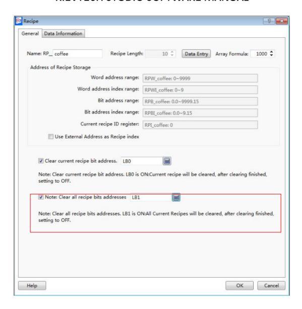
For the above example, all the data of the recipe "RP\_coffee" will be cleared if the bit register LB1 is ON. After the data is cleared, LB1 will be reset OFF.
