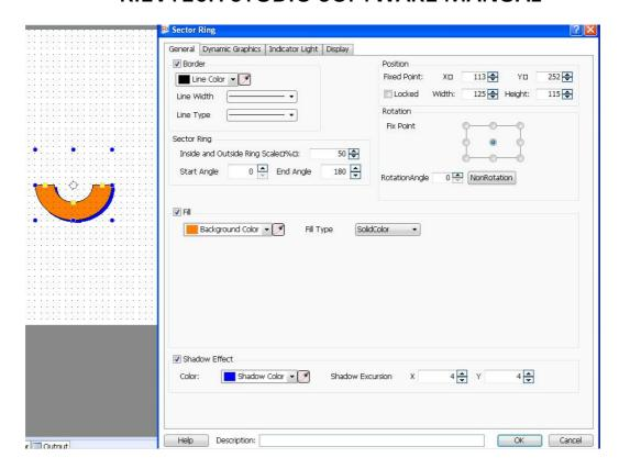
A sector ring can be got by setting the properties such as line color, line width, line type, starting angle, end angle, position, rotation, fill color, fill type and shadow effect. It can be freely drawn by dragging the yellow and blue areas.
