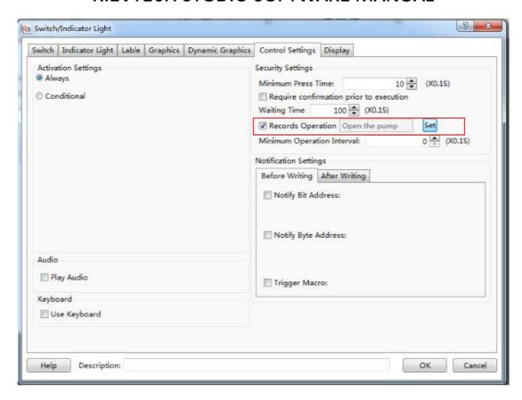
If you check this function, you can record the operations of the component and display the records in the operator Log. It is shown as below.
