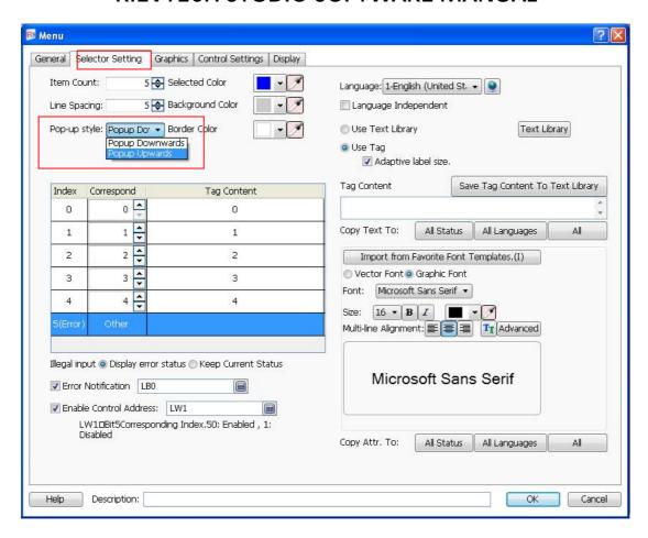
For "The Drop-down List" component, the most settings of the "Selector Setting" property TAB are same to the "Check list and selection boxes". The difference is that there is an additional item of "Pop-up style" for the "The Drop-down List".
