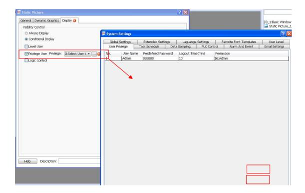
Logic Control: The static picture visibility can be controlled by the address conditions. The conditions include bit control (address ON and OFF) and word control (word address value conditions).
