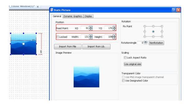
The static picture size and position can be fixed if the "Locked" is checked. And the static picture can be rotated around a fixed point. The fixed point and rotation angle can be set. The picture can be manually rotated (in any angle) after the fixing angle is set.
