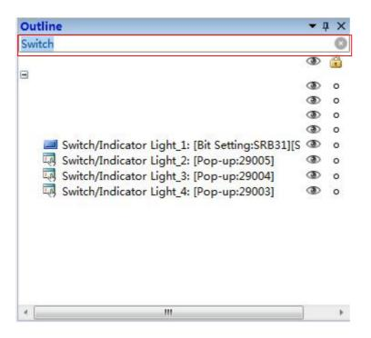
When you click the little eye tool " " except the top one, it will change to " " and hide the corresponding component in the window. When you click it again, it will change to " " and make the corresponding component show in the window. The top little eye tool " " will control all components hide or shown by clicking it.
