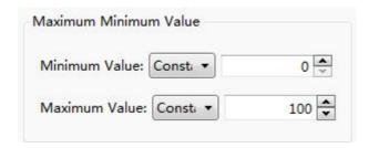
If you select by Variable, you can specify a word register and enter a value to the word register to change meter during running your project, as shown in the figure below.
