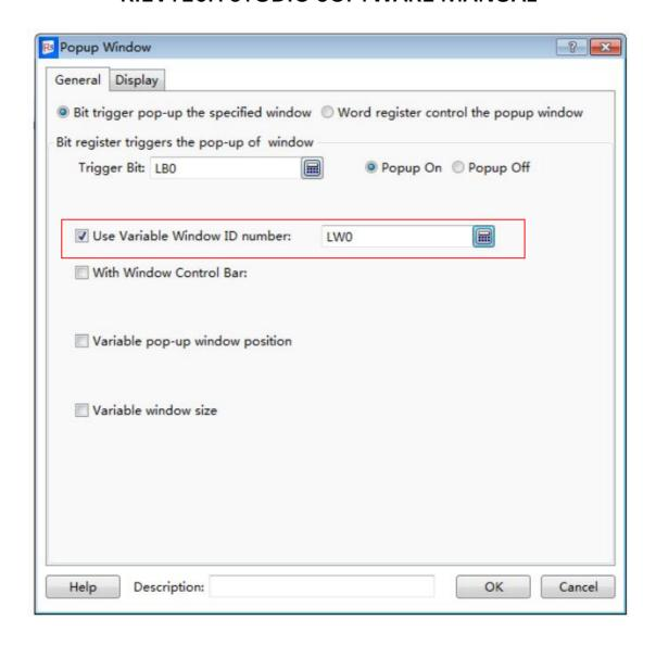
For the above example, the word register is specified LW0 and a numeric value input component connected with LW0. The simulation running result is shown as below. Enter the corresponding window ID number in the numeric value input component and then click the button "Popup the window", the designated window will pop up.
