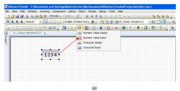
ow(1)\* × Numeric Input General Number Format | Keyboard Setting | Font | Graphics | Dynamic Graphics | Control Settings | Display Operation Attribute: Numeric Display Numeric Input Characters Display Characters Input 1234 Reading And Writing Address Is Different Password Read Address: Use Address Tag Deivce: LOCAL:[Local Register] Address Type: LW Address: 0 Format(Range) DDDDD(0~7... Occupy: 1 - Word Address Index Set the variable address Help Description: OK Cancel
