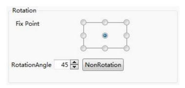
The function of "Rotation" can adjust the display angle of the components such as static graphics, vector graphics and other components. This function is a static function. That is, the display angel is not adjusted in the HMI if you set the display angle in the "Rotation" property. If you want to dynamically adjust the display angle of the graphics, please refer to: <a href="Detailed manual/General functions/Dynamic Graphics">Detailed manual/General functions/Dynamic Graphics</a>.
