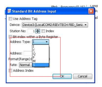
If the address is not connected with the device after you input a specific address number, you should check whether the parameters (such as Device, Station No. and Address) are set correctly. For example, these parameters a reset as follows.
