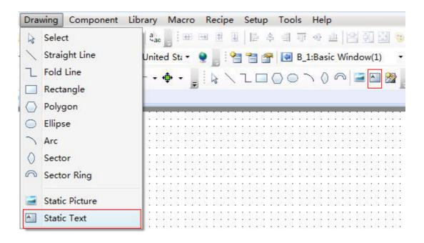
When click the Static Text command, the properties dialog will pop up. The content of the static text to be displayed can be written into the Tag Contents. The font, size, color and alignment mode can be set here.
