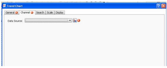
In the "Channel" property TAB, you need select a sampling data as the "Data Source". There will be a red exclamation mark here if the "Data Sampling" is not set. You can open the "Data Sampling" settings page to set the required sampling data by click the button
