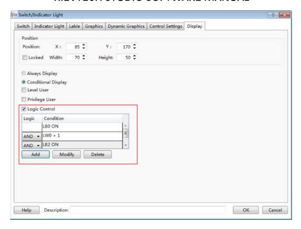
If you check this function, the component can be controlled to display according to the logic condition. The condition can be multiple logical operations.
