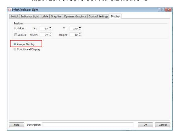
If you select the "Always Display" function, the component will always be visible when the project is running. It is the default setting.
