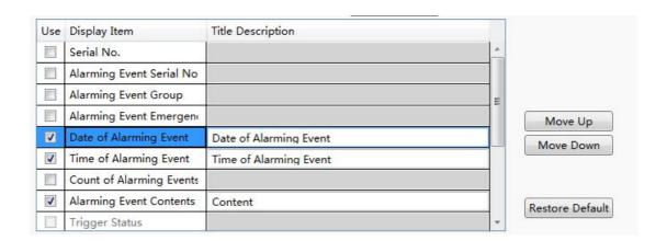
You can use the button "Move Up" or "Move Down" to modify the order of the display items arrangement. The content on the toprow will display on the left of the alarm bar. You can restore the default arrangement by clicking the button "Restore Default".
