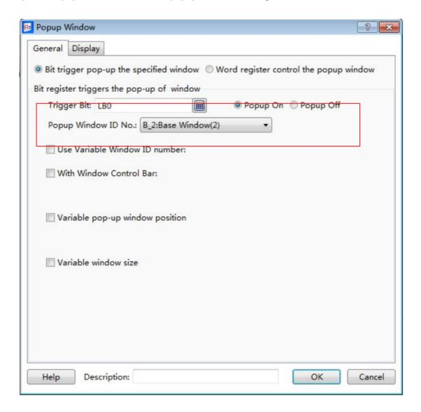
For example, a button named "Popup the window" is connected with LB0 and the trigger bit of the popup window component is set LB0. The simulation running result is shown as below. When press the button "Popup the window", the specified window will pop up.
