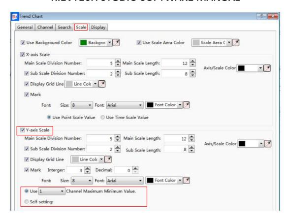
After you select the option "Use ... Channel Maximum Minimum Value", you can specify a channel number. And the minimum and the maximum values of this channel will be used as the minimum and the maximum values of the Y axis.
