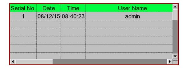
You can hide the grid line if you don't check the "Row Split Line" and the "Column Split Line". It is shown as below.
