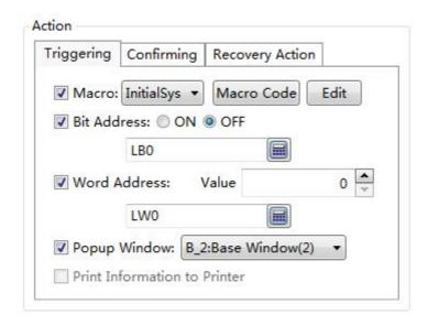
The actions of "Triggering" refers to the actions that they will be executed when the alarm or event occurs. The actions of "Confirming" refers to the actions that they will be executed when the alarm or event is acknowledged by manual. The actions of "Recovery Action" refers to the actions that they will be executed when the alarm or event exists.
