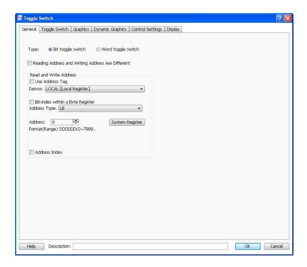
The "Bit Switch" component can be found on the tool bar or from the menu of Components.
