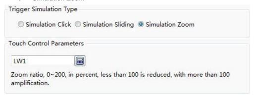
When the trigger conditions of the touch trigger component are met, the components which occupy the active area of the touch trigger component will execute the zooming action within this area, such as viewing the trend curve by zooming.
