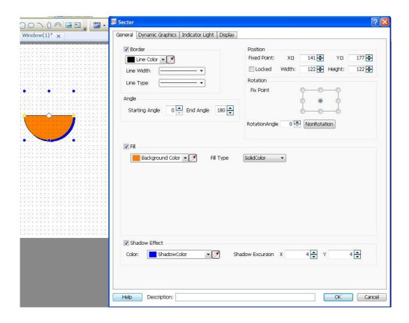
A sector can be got by setting the properties such as line color, width, type, starting angle, end angle, position, rotation, fill color, fill type and shadow effect. It can be freely drawn by dragging the yellow and blue areas.
