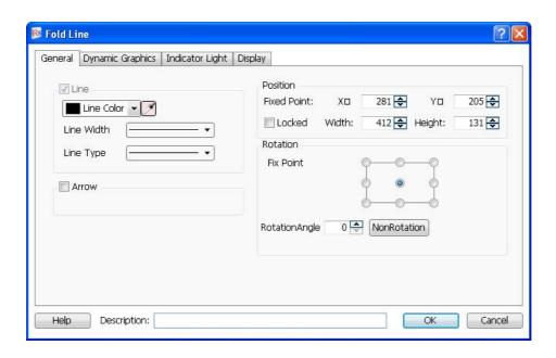
Click the left key to fix the fold line point in drawing. And click the right key to finish drawing. See details in: <u>Detailed Manual/ Drawing/ Straight Line</u>.
