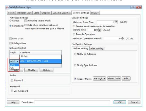
There are the button "Modify" and the button "Delete" besides the button "Add" in the Logic Control list. After selecting a condition in the Logic Control list, you can click the button "Modify" to edit it again or click the button "Delete" to remove it from the Logic Control list. You can also double-click a condition in the Logic Control list to modify it.
