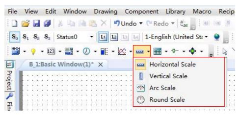
The "Horizontal Scale" is mainly used to display a progress bar. The "Vertical Scale" can be used to display the current liquidlevel of a tank orthe charge state of a battery. The
