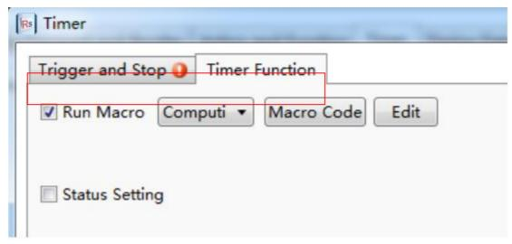
In this example, executethe "Computing" macro when the input value changes by using the timer function. See settings as shown as below. The detailed using method of the timer component, please refer to: <a href="Detailed manual/Component/Timer and Data">Detailed manual/Component/Timer and Data</a> Transmission/Timer.
