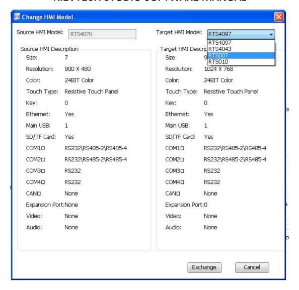
After you select the "Target HMI Model" for your project and click the button "Exchange" to confirm the setting, the project will be converted to adapt the new HMI device.
