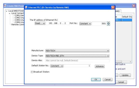
(c) Ethernet PLC (Or Service by Remote HMI)
