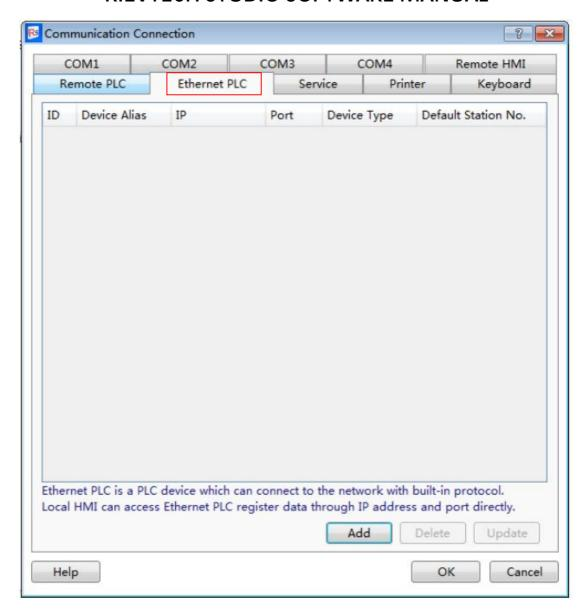
After click the button "Add" in the "Ethernet PLC" settings page, the "Ethernet PLC" settingsdialog will pop up. It is shown as below.
