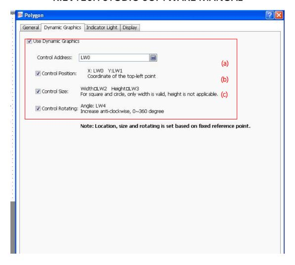
(a) Position control (b) Size control (c) Rotation control
