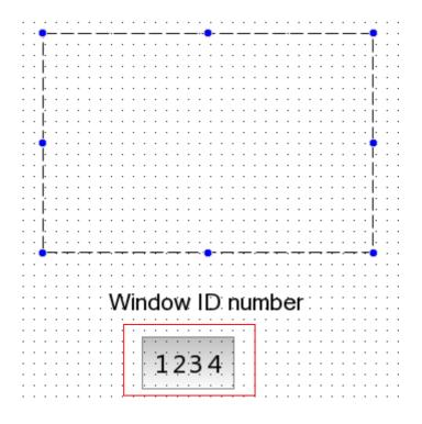
The simulation running result is shown as below. When input a positive integer value to the numeric value input component, the window which the ID number of it is equal to the inputted value will pop up.
