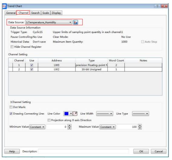
After you selecting a sampling data for the option "Data Source", all channels of this sampling data defined in the "Data Sampling" will be displayed in the "Channel Setting" property box.
