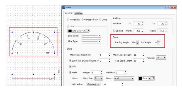
For the option "Position" in the "Scale" property box, the axis position of the sacle can set "In", "Out" and "Center".
