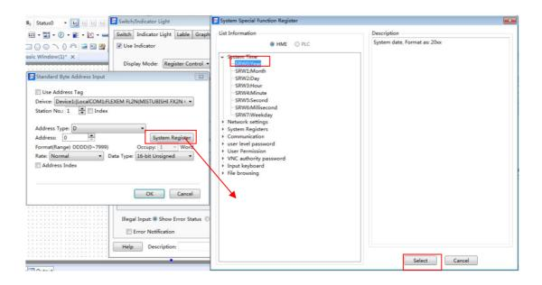
Certainly, the screen is connected with multiple slaves at sometime. The station number is varied. At this moment, you need to use the Index function. This function uses a byte or word address to provide a variable station number. The setting process is shown as follows.
