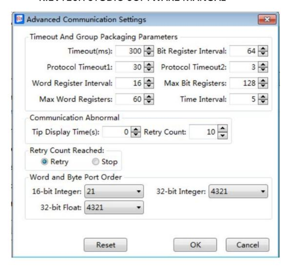
The parameters in the Advanced Communication Settings should not be modified, unless the professional guidance is given. The optional modification may result in a communication failure or unexpected events occur. You can consult the factory technical staff to modify the advanced parameters based on your needs. In most cases, the default parameters are the bestand neednot to be changed.
