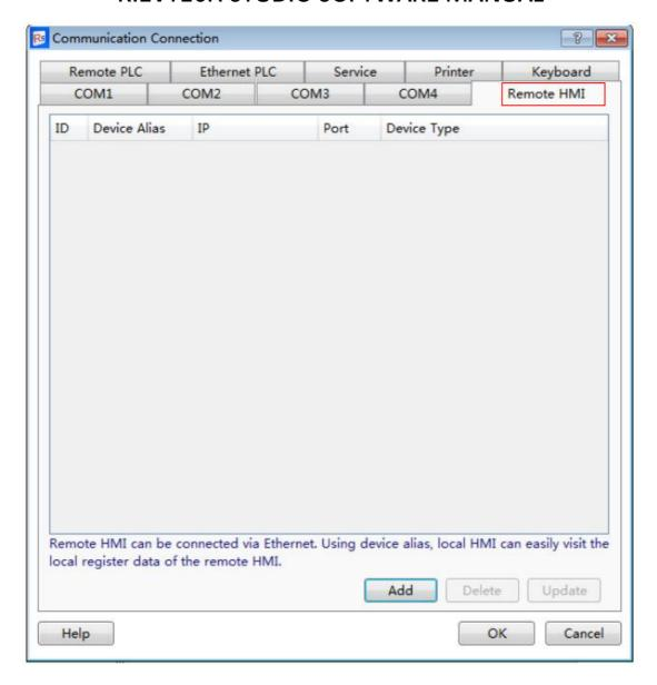
For one of the HMI device, anyone of other HMI devices in the same Ethernet network of the LAN is the Remote HMI. For example, there are two HMI: one named HMI1, another one named HMI2. These two HMI devices are connected an Ethernet network. For HMI1 device, HMI2 is the "remote HMI" of HMI2. For HMI2 device, HMI is the "remote HMI" of HMI2.
