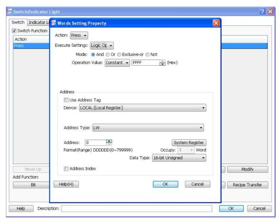
In the figure above, when the component is operated, the value in register LW0 will has a logic operation"And" with 0×FFFF. The logic result will be written to register LW0. The operations of otherthree modes are similar to "And" mode but the logic operation.
