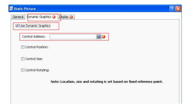
When the control address is fixed, the position, size and rotation can be controlled. E.g.: when there are many sector pictures, they can be set to display rotating effect by setting the Control Rotating.
