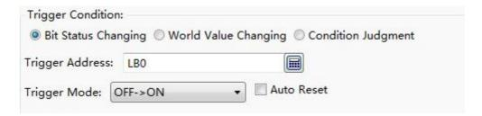
The "Trigger Condition" supports "Bit StatusChanging", "Word Value Changing" and "Condition Judgment". The settings are referred to: <a href="Detailed manual/Component/Timer">Detailed manual/Component/Timer</a> and <a href="Data Transmission/Timer">Data Transmission/Timer</a>.
