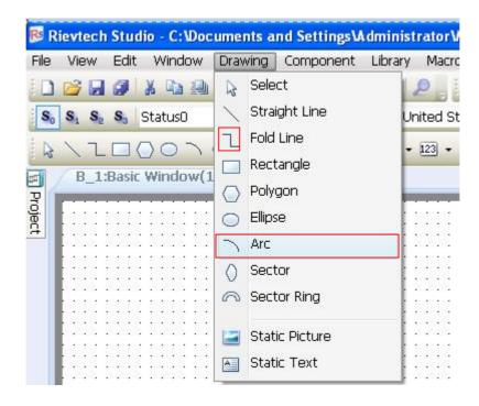
Select the arc component, designate any area to draw, and double click to set the arc properties.
