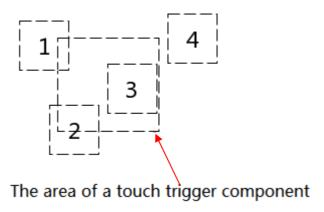
As shown as above, when the trigger condition of the touch trigger component is met, the components 1,2 and 3 will be triggered, while component 4 will not be triggered.
