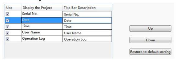
You can select the required contents to display in the title bar by checking in the "Use" column. For the order of the contents arrangement, you can use the button "Up" or "Down" to modify it. The content on the toprow will display on the left of the Operator Log List. You can restore the default arrangement by clicking the button "Restore to default sorting".
