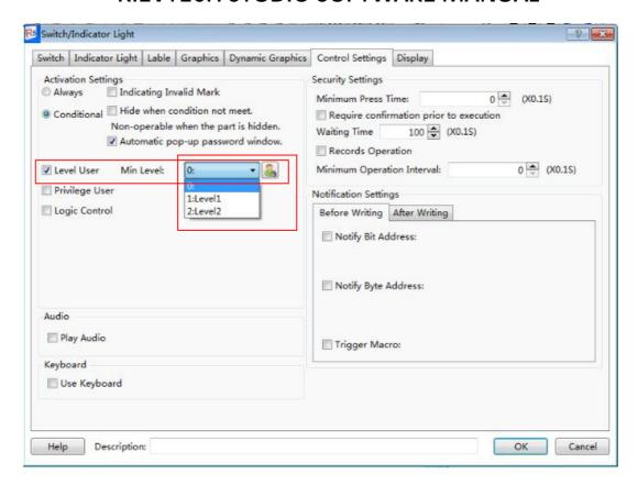
Run the project. A "User level login" window will pop up when you click the component. It is shown as below. You can operate the component only by entering the correct password in the "User level login" window.
