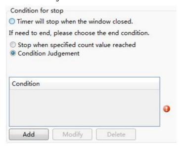
You can control the timer to end by using a set of conditions. When the conditionsaresatisfied, the timer execution ends. For the logical condition editing, see: <a href="Detailed manual/General functions/Drawing/Logic Control">Detailed manual/General functions/Drawing/Logic Control</a>.
