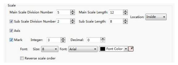
You can set the "Main Scale Division Number", the "Main Scale Length" and the "Sub Scale Length" here. The Location of the scale can be set "Inside", "Outside" and "Center", as shown as below. The "Sub Scale Division Number" and the "Axis" are checked by default. The default sub scale division number is 2. If the "Sub Scale Division Number" and the "Axis" are unchecked, that means the sub scale and axis are not displayed.
