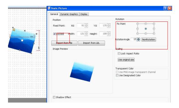
The static picture size can be set in the properties window by the Scaling function. It can be set either by checking "Lock Aspect Ratio" (the fixed horizontal/vertical ratio) or by checking "Use original size" (keeping the original size).
