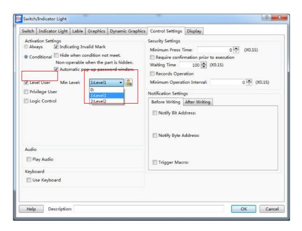
After checking this function, you need to enter the appropriate user level password to operate the device. It is shown as below.
