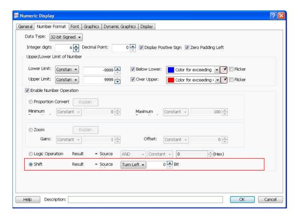
The data can be shifted left or right by the component. And the result of shifting operation will be displayed.
