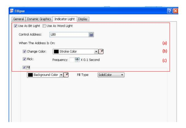
(a) Modify the frame color (b) Control flickering frequency (c) Modify the filling color
