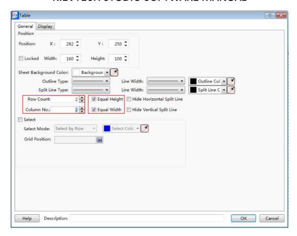
The option "Hide Horizontal Split Line" and the option "Hide Vertical Split Line" can be checked. You can check anyone or two to hide the split line of the table according to your needs
