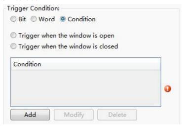
If you select "Condition" option, you can use a set of conditions to control the timer trigger. For the logical condition editing, see: <a href="Detailed manual/General">Detailed manual/General</a> functions/Drawing/Logic Control.
