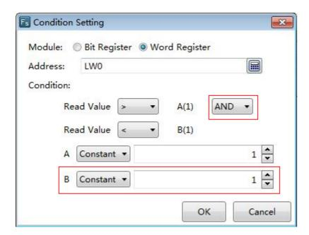
If the conditions you need is "LW0> 100" and "LW0 <LW1", then the condition of the second is not "constant" but "variable" and the address is LW1. The setting is shown as below.
