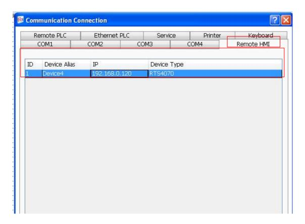
Click the button "OK" in the "Remote HMI" settings page to save, and then you can find the remote HMI device in the Device list of the register address. For example, it is shown as below.
