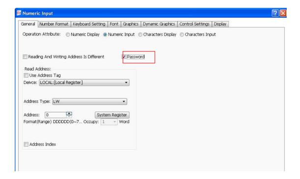
When the "Password" is checked, "\*" will be displayed in the component (See the figure below). It can be checked if the current component is used to input the password.
