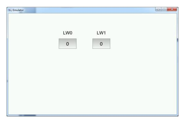
Input the value 100 to LW0. The output value of LW1 will be 300 according to the rules that the output value will be 3 times as much as the input value if the input value is less than or equal to 300.
