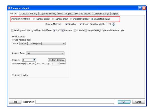
The "Operation Attribute" includes four operation types: "Numeric Display"," Numeric Input"," Character Display" and "Character Input". If you want the current Character Input component change to the Character Display component or Numeric component, you can modify it here. It is highly efficient for the project modifying and maintaining.
