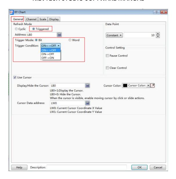
For example, if the trigger condition is set "OFF→ ON", that means the XY curve will be refreshed when the specified bit register is changed from OFF to ON.
