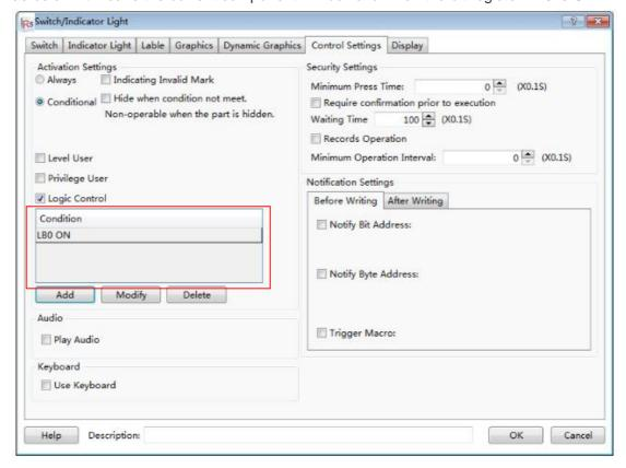
If the condition is not enough, you can continue to add. For example, the condition "LW0 > 1" need to be added. You can click the button "Add" to go on the operation. The Word Register is selected and the address is set LW0. The condition is set "LW0 > 1". The setting is shown as below.
