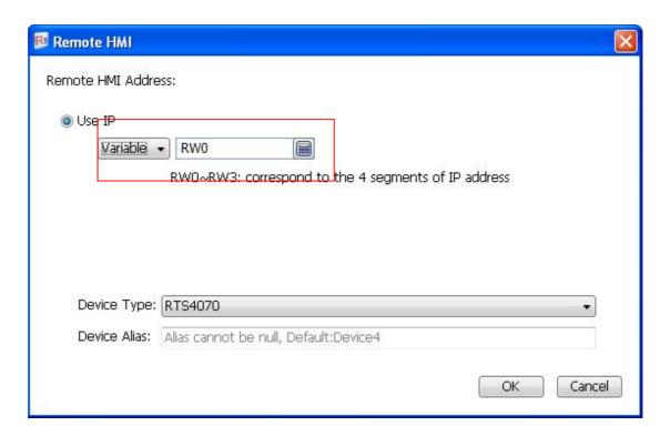
You can input the IP address of the Remote HMI to the4 word registers by the numeric value input component. Then you can access the desired HMI device.
