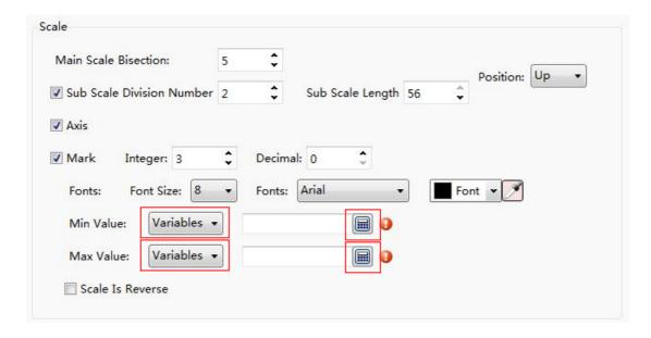
Usually, the scale value is displayed increasing from left to right. Sometimes, it needs to be displayed increasing from right to left. To do that, you should check the option "Scale Is Reverse".
