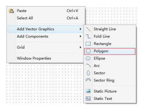
A side will be added every time when the left key is clicked. After all sides are obtained, a polygon can be obtained by clicking the left key and then clicking the right key.
