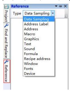
For example, all the uses of "Data Sampling" in the current project are listed in the following after select it.
